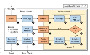
Fig. 1: Transformation of sandbox macro. The angled orange boxed are SDRaD functionality, while rounded blue boxes are new glue logic for parameter passing and error handling.
